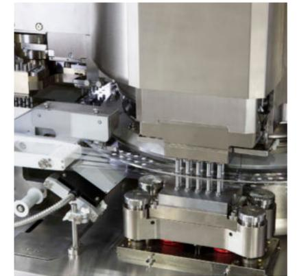
Our tablet press achieves high accuracy and high efficiency production in all stages, from supplying precise amounts of material to pressing, inspection, sorting, and drying.
