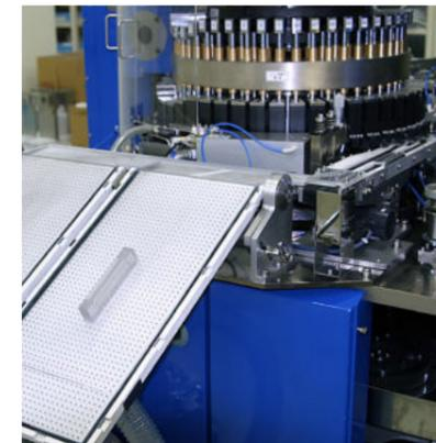
This assembly machine makes small, coin-cell consumer-use batteries. It makes full use of Sankyo cam technology.
