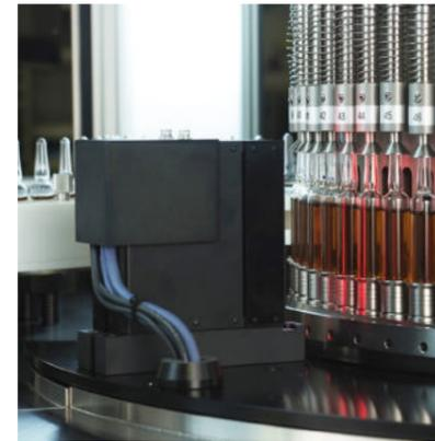
The ampoule inspection supply mechanism uses an indexing device developed by us. It has been adopted in ampoule inspection machines around the world.
