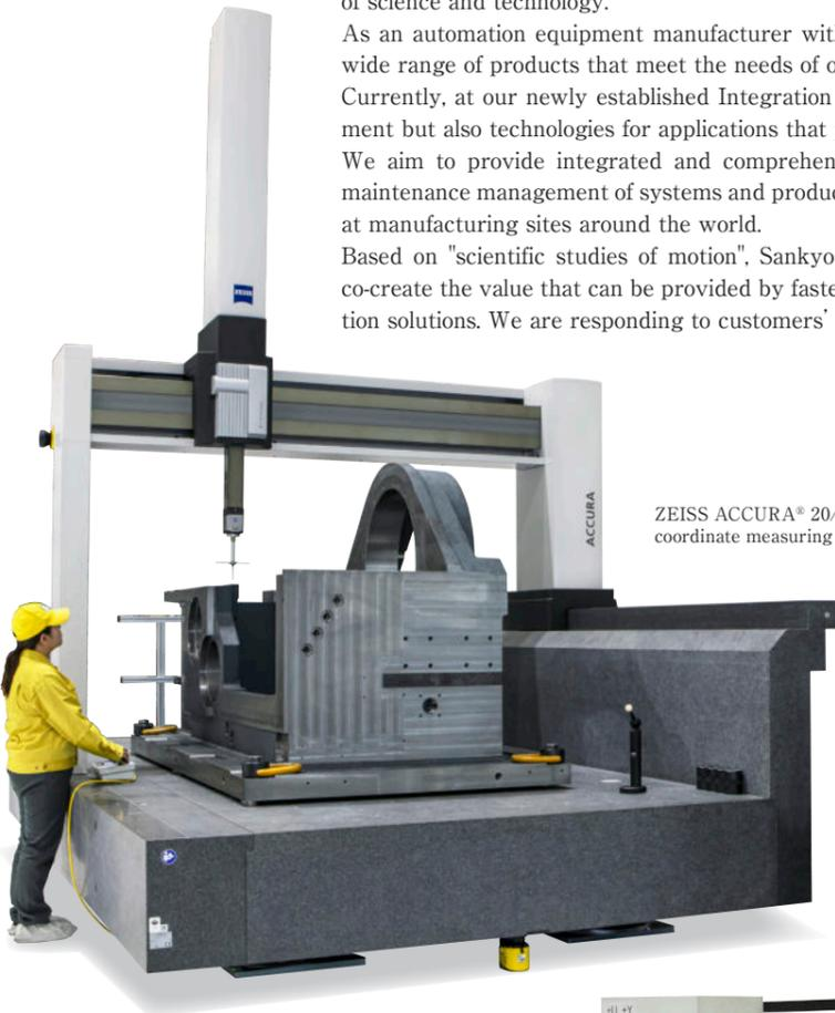
ZEISS ACCURA® 20/42/15, very large, three-dimension, coordinate measuring machine
